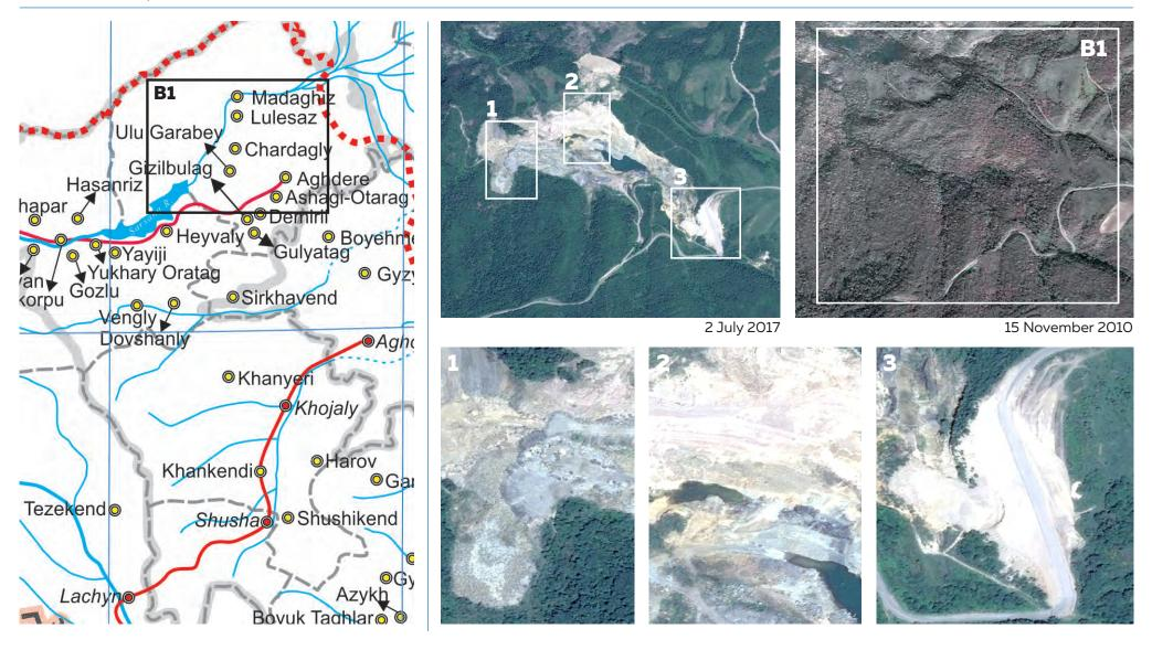
2. Mining and ore processing facilities on 253.32 hectares of copper-molybdenum mine near Demirli village in the occupied part of the Tartar district | 40° 09' 03" N, 46° 47' 21" E
